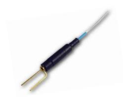
The Tap Optical Power Monitor is a hybrid fiber optical passive component that integrates a thin-film tap of flat spectral response with a high sensitivity PIN photodiode for power monitoring applications. The Power Monitor minimizes component assembly costs and module footprint while increasing module design efficiency by facilitating fiber Management.
